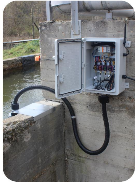
(1) Watertight ABS box; (2) Radio antenna; (3) Power; (4) Air sensors; (5) Water quality sensors connection; (6) Ultrasound sensor connection; (7) Ultrasound sensor; (8) Water quality sensors container
