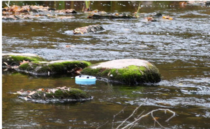
Figure 1. First prototype of the Smart Geo Particle drifting in the Pirita River.
